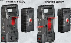
NOTE: To ensure a good connection between battery and RED™ CHARGER, RED CRADLE, RED QUICKPLATE, and/or RED BATTERY PLATE V-plate adapter, it is recommended to perform a break-in sequence. **To break-in:** Fully engage/disengage a RED BRICK battery approx. 20 times in V-plate adaptor.
